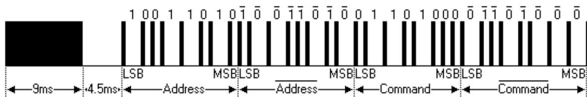
A command is transmitted only once, even when the key on the remote control remains pressed. Every 110ms a repeat code is transmitted for as long as the key remains down.
